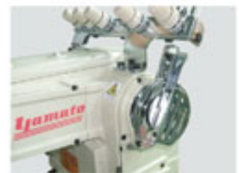
external thread take-up thread is supplied smoothly
