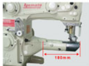
cylinder length: 180mm easy to load/unload the fabric
